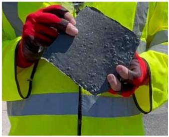
The material will accommodate that movement without cracking. It will stay stuck to the surrounding concreteand will not crack. Making it the perfect material for sealing concrete cracks and joints. Once applied to the surface it is dressed with a bauxite aggregate finish to give skid resistance and a yellowed colour finish.
