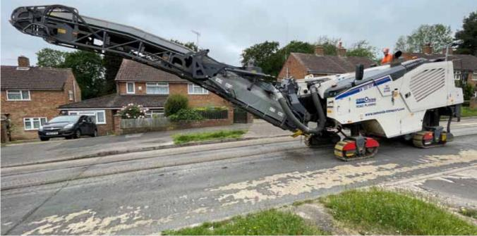
The midrange tracked machine with a 1.2 metre cut. The drum at the rear and elevator at the front makes it ideal for smaller jobs, estate roads and car parks but also capable of larger jobs when necessary.
