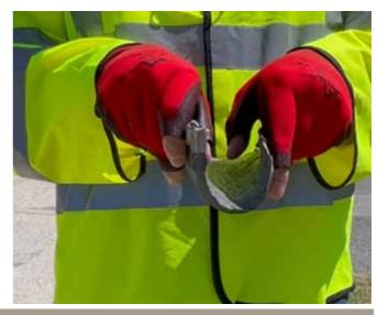
The joint repair material is a synthetic binder with a high polymer content and aggregates. The material is very flexible making it able to accommodate the high movement typically found at a concrete joint without cracking
